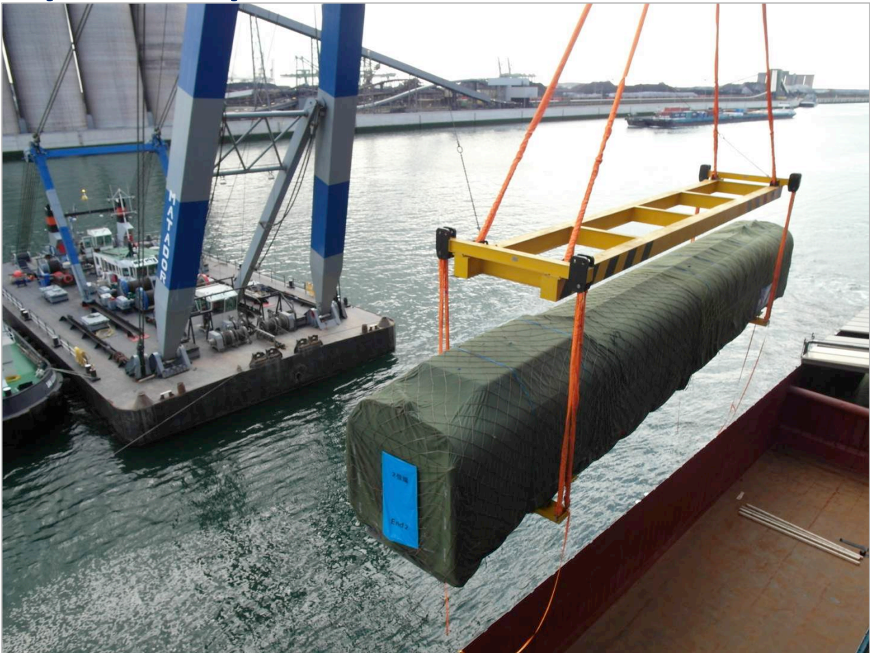
Loading of second tain into the barge.
